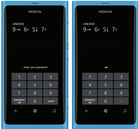
Figure 1. The device and the custom application used during the study. The first picture illustrates the initial state of the hybrid condition, where a random hybrid password 9→ 6° 5↓ 7° was generated by the system. The password can be located at the top of the application. Here, to unlock the device, one has to make a left gesture on the “9” key, tap on the “6” key, make a down gesture on the “5” key, and then tap on the “7” key. The second picture illustrates a state where a user already inputted the first two items. Note that, here and similar to the default Windows Phone 7 lock-screen, the “cancel” button has changed to the “backspace” (⌫) button to accommodate error correction.
