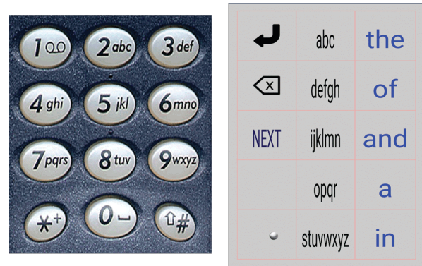
Figure 2: Inspired by the T9 technique (left), TiltWriter also implements a Custom ambiguous keyboard (right).
