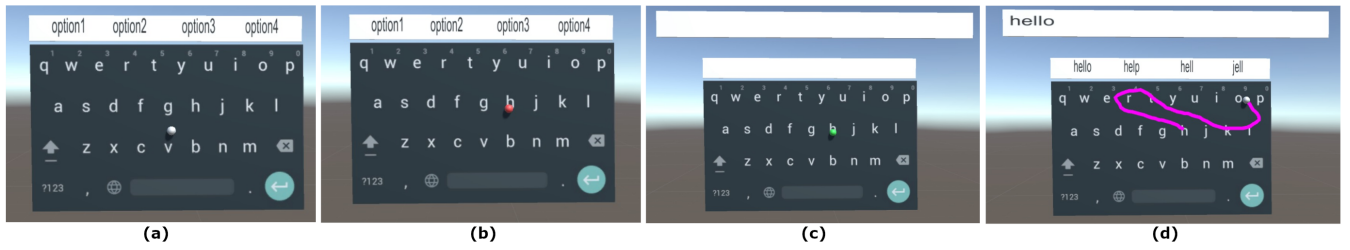
Figure 4: Shapeshifter looks and feels like the default Google Android keyboard. To enter text with Shapeshifter, the user (a) touches a surface (grey cursor), (b) applies extra force to activate the cursor (red cursor), (c) positions the cursor over the first letter of the intended word and applies extra force to start a gesture (green cursor), and (d) completes the gesture maintaining extra force, then reduces force to automatically enter the word associated with the gesture (pick tracing). Shapeshifter enables users to enter multiple words by switching between regular and extra force, without ever lifting the finger. Lifting the finger off the surface deactivates the cursor. The keyboard displays a suggestion bar with the most probable alternative words. The user can replace the output word with a suggested word by applying extra force upon moving the cursor over the suggested word, like pressing a button.
