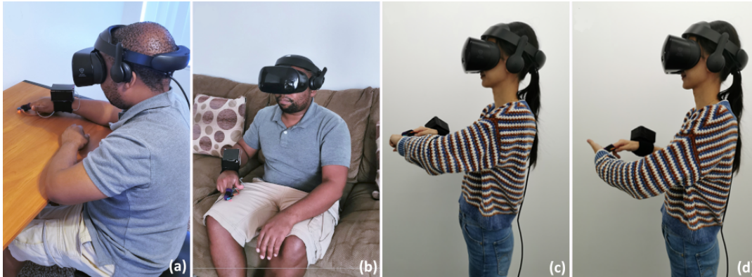
Figure 1: Two users using Shapeshifter to gesture type in virtual reality in four scenarios: (a) on a desk when sitting down, (b) on the lap when sitting down, (c) on the back of the hand when standing up, and (d) on the palm when standing up. Both users are wearing the digital thimble introduced in this paper for gesture detection.
