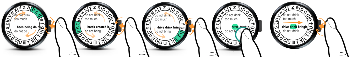
Figure 6: The process of entering the word “drink” with manual Crownboard. The user rotates the crown upward to scan the zones in clockwise direction. When the key with the letter ‘d’ is highlighted, she presses the crown to select it. The user then rotates the crown downward to scan the zones in counterclockwise direction, selects the zone containing the letter ‘r’, then continues scanning in the same direction to select the zone containing ‘i’. The user notices the target word in the suggestion bar. She taps anywhere on the screen to start scanning the suggested words by rotating the crown, then selects the intended word by pressing the crown.
