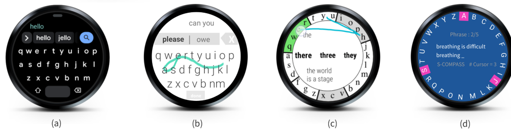
Figure 3: The four existing smartwatch techniques demonstrated in the focus group: (a) Wear OS QWERTY [10], (b) WatchWriter [29], (c) SwipeRing [78], and (d) COMPASS [96].
