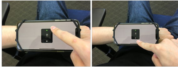
Fig. 2. Input stepper is the default number picker on most smartwatches: it displays a full-screen number wheel that users spin by flicking up or down to increment or decrement a numeric value, respectively.
