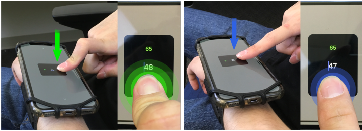
Fig. 5. Force-based number picker: the user applies extra force to increment and soft force to decrement a numeric value.
