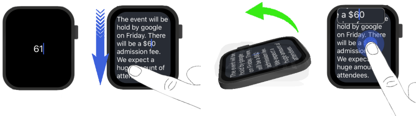
Fig. 1. The four number pickers investigated in this work, from left: input stepper (the default number picker on most smartwatches), swipe (in this figure, the user is swiping down to decrease a value), tilt (in this figure, the user is tilting up to increase a value), and force (in this figure, the user is varying contact force to change a value). Unlike the default input stepper, the new methods do not display numeric values in full-screen when selected, instead display a magnifier window to display the value changing (see the last image).
