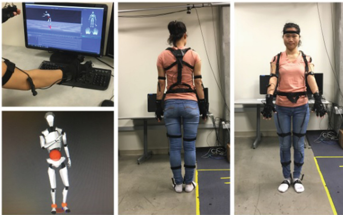
Fig. 3. Perception Neuron full-body motion capture suit setup
